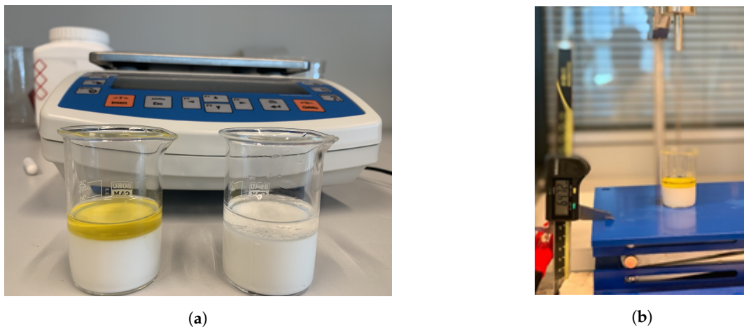
Figure 3. Double-layered configurations and part of the experiment setup for the measurement of layer thickness and step size: (a) skin phantom-olive oil (left) and skin phantom-triton X-100 (right), (b) adjustable stand and digital caliper for thickness measurements.
