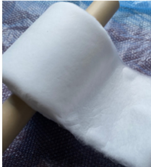
Figure 15. Meltblown nonwoven fabric sheet which was made of degraded PP by high-shear extruder. We used PP2 as the raw material because no talc was included as the additives.
