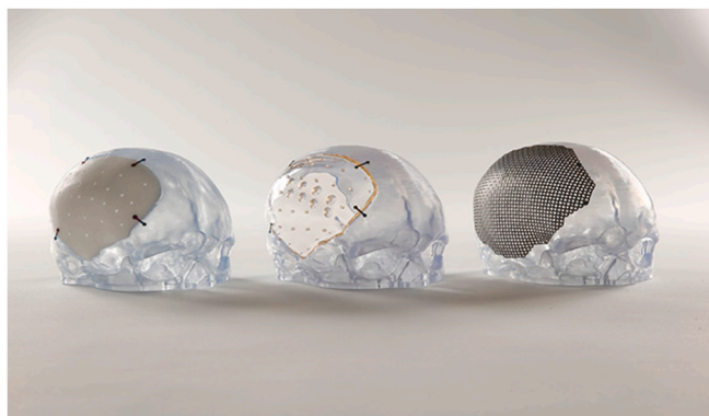
Fig. 1. Cranial Biomodel with a patient-specific implant in situ. Implants are made from (Left) Porous high-density polyethylene (StarPore®), (Centre) Polymethylmethacrylate, (Right) Titanium mesh.
