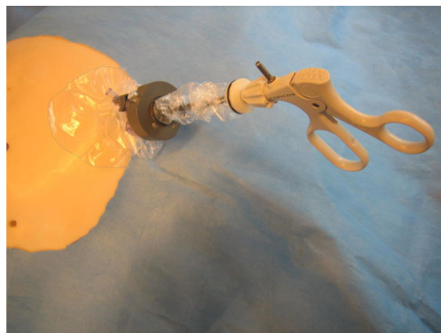
Fig. 6 Dexterity test setup: instrument handling was tested on a plastic model of the inflated abdominal area
