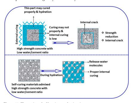
Figure 11. Illustration of self-curing mechanism in concrete.
