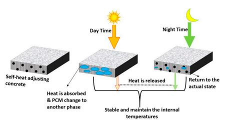
Figure 15. Schematic diagram of the mechanism of self-temperature adjusting concrete [310].
