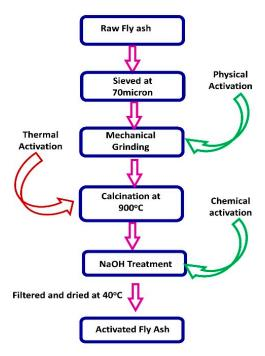
Figure 2. Schematic diagram for fly ash activation process.
