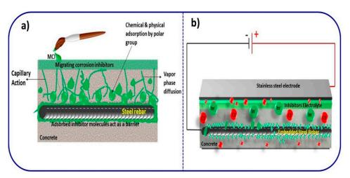
**Figure 10.** Schematic diagram of the migrating (a) and electro-injection (b) methods of corrosion inhibition.
