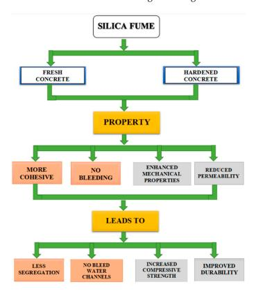
Figure 5. Schematic of mechanistic action of SF in fresh and hardened concrete.
