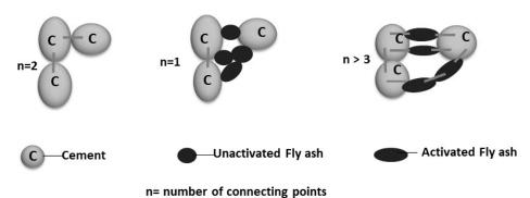
Figure 3. Binding mechanism of activated and inactivated fly ash.
