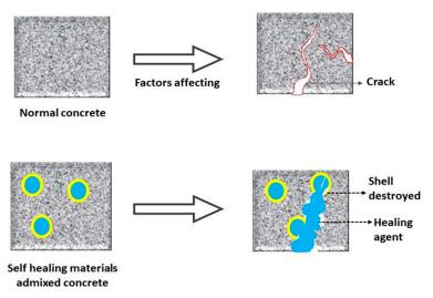
Figure 12. Illustration of the self-healing mechanism in concrete.
