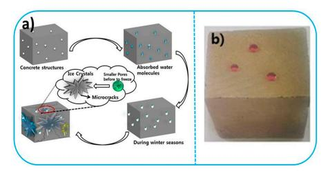
**Figure 13.** Schematic diagram of the mechanism of crack formation in concrete (a); Incorporation of hydrophobic materials admixed in concrete (b) [255].
