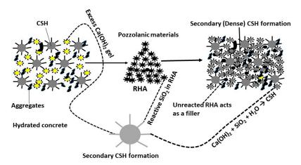
**Figure 7.** Hydration process for cement with the addition of RHA.
