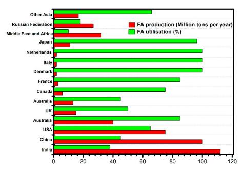
Figure 1. Worldwide production and utilization of fly ash and source data from [11].
