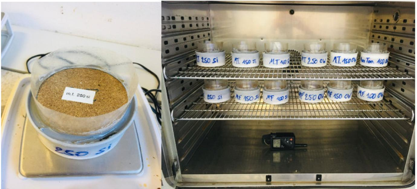
**Figure 3.** Embedded specimen (dry cup/wet cup).
