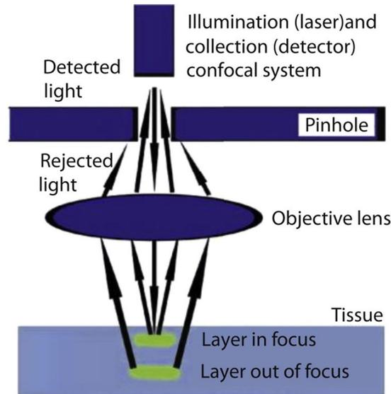
**Figure 1.** Schematic diagram of confocal laser endomicroscopy principles.<sup>33</sup>
