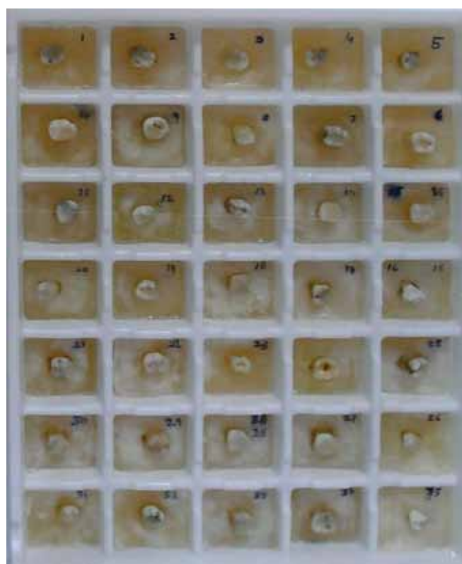
Fig. 2: Prefabricated template bearing samples for scanning
