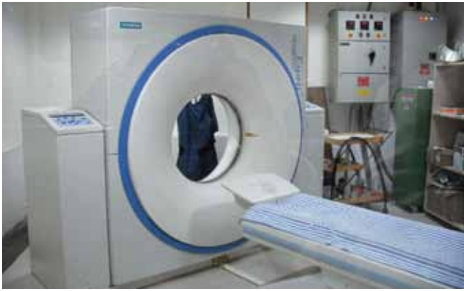
Fig. 3: Spiral computed tomography unit (Siemens® SOMATOM Esprit + CT)
