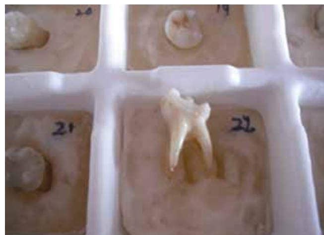
Fig. 1: Sample embedded in acrylic jig permitting accurate repositioning
