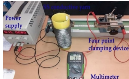
Figure 3. Measuring of length-dependent resistance (four-point clamping device).
