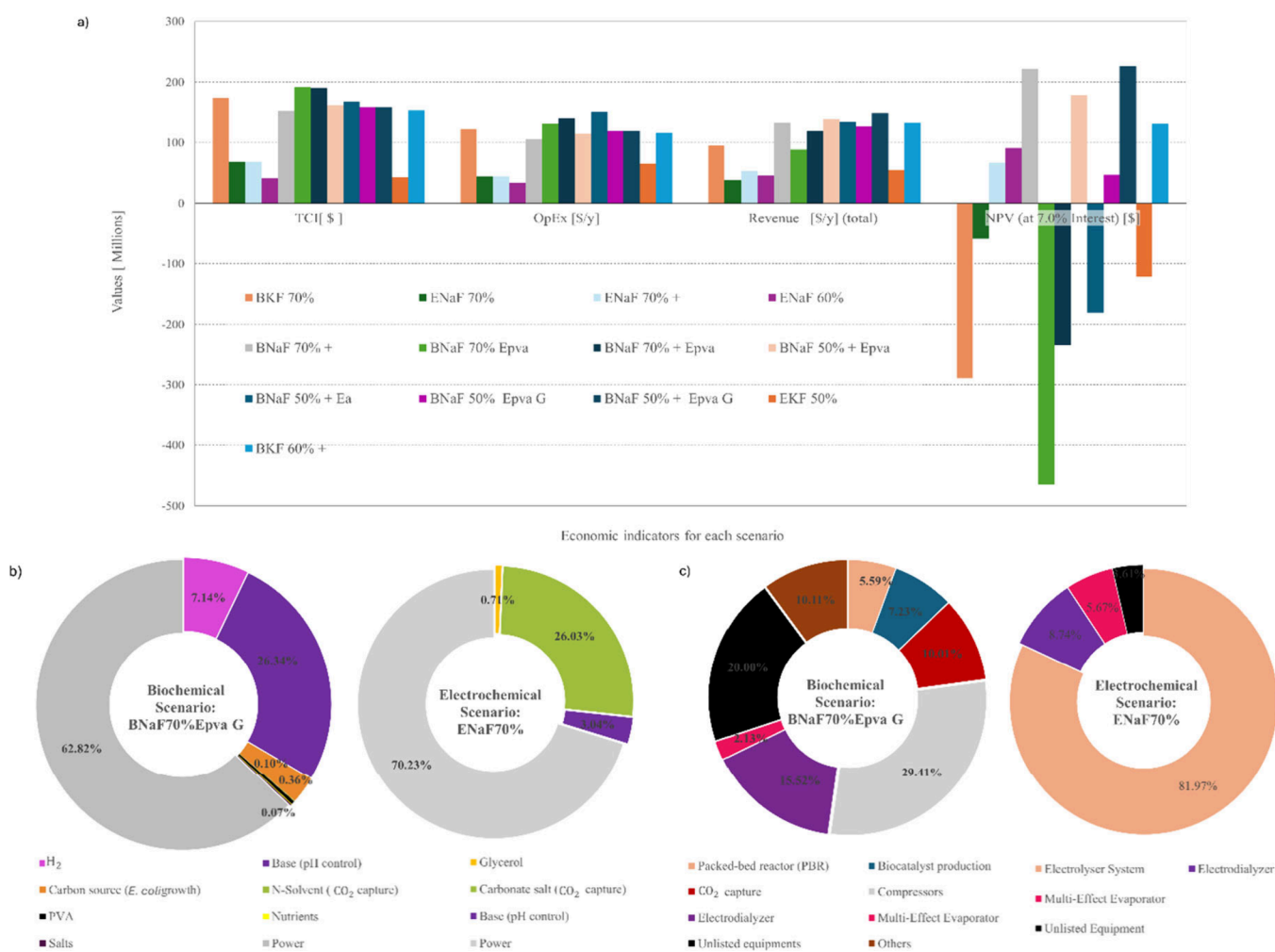
Figure 1. Techno-economic analysis. NPV, TCI, revenue, OpEx, and CapEx (a). Breakdown of OpEx (b) and CapEx (c). Additional income from BFG treatment was indicated by the + sign. E PVA and E a indicated immobilization in PVA and alginate supports, respectively. Glucose (G) and formate-CO 2 (CCU) were used as the carbon source for bacteria growth.
