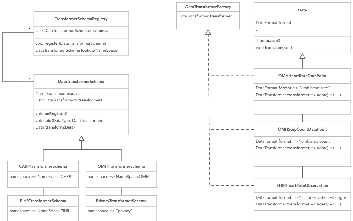
Figure 3. The UML class diagram of the ‘Data Transformer’ pattern with the HR data from the Movisens device being transformed into the OMH and FHIR data formats as an example. *: Multiplicity.
