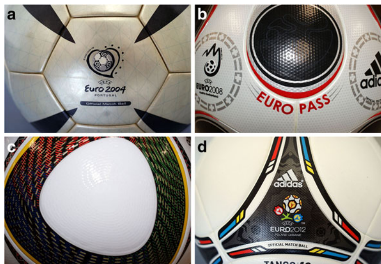
Figure 1 Photographs of soccer balls. (a) Adidas Roteiro: smooth surface with 32 pentagonal and hexagonal panels. (b) Adidas Teamgeist II: small protuberances with 14 panels. (c) Adidas Jabulani: small ridges or protrusions with 8 panels. (d) Adidas Tango 12: small grip texture with 32 modified panels.
