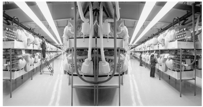
FIGURE 21.6 Gnotobiotic facility utilizing flexible film isolators. Courtesy Charles River Labs.
