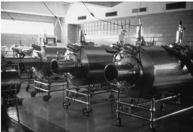
FIGURE 21.5 Stainless-steel isolators. Courtesy University of Notre Dame.
