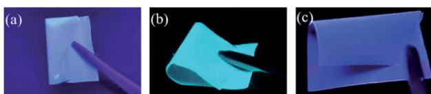
Fig. 10 Images of renewed polyimide films under 365 nm ultraviolet light (a) PI(PBAI-CBDA), (b) PI(MPBAl-CBDA), (c) PI(TFPBAI-CBDA).
