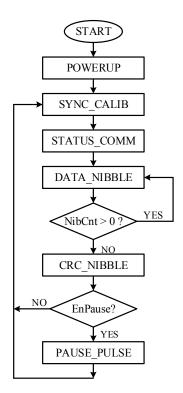
Figure 5. SENT main controller flow chart.
