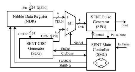
Figure 4. Proposed SENT transmitter architecture.
