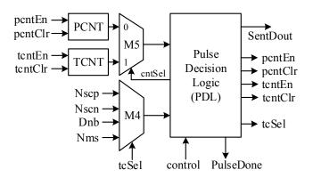
Figure 10. SENT pulse generator architecture.
