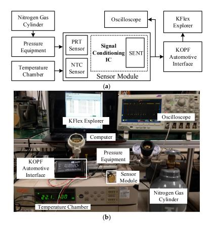
Figure 15. Measurement setup. (a) Measurement setup block diagram; (b) Measurement setup lab setup.
