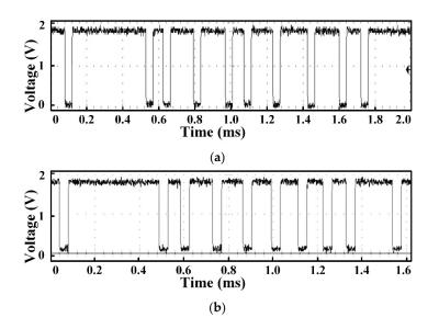
**Figure 19.** SENT measurement result. (**a**) Data (9A18CA)<sub>16</sub>, CRC (3)<sub>16</sub>, clock ticks 205, duration 1.640 ms; (**b**) Data (654321)<sub>16</sub>, CRC (E)<sub>16</sub>, clock ticks 187, duration 1.496 ms.
