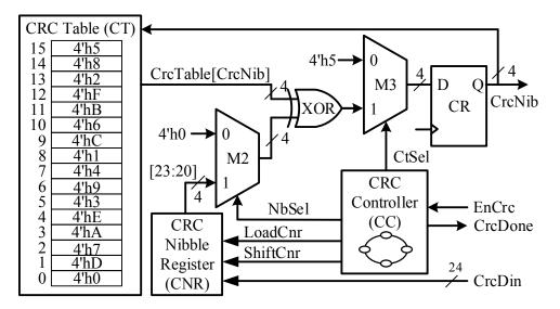
Figure 7. The SENT CRC generator architecture.
