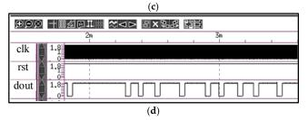
**Figure 14.** SENT simulation results. (**a**) CRC calculation with data  $(2A9D6B)_{16}$  and CRC  $(D)_{16}$ ; (**b**) Data  $(2A9C63)_{16}$ , CRC  $(B)_{16}$ , Clock Ticks 228, Duration 1.824 ms; (**c**) Data  $(F37D91)_{16}$ , CRC  $(1)_{16}$ , Clock Ticks 201, Duration 1.068 ms; (**d**) Data  $(4CD163)_{16}$ , CRC  $(B)_{16}$ , Clock Ticks 207, Duration 1.656 ms.
