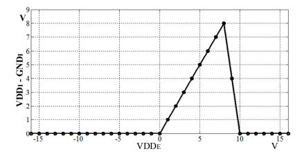
Figure 21. Reverse and over voltage protection measurement result.
