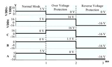
Figure 20. Reverse and over voltage protection simulation result.
