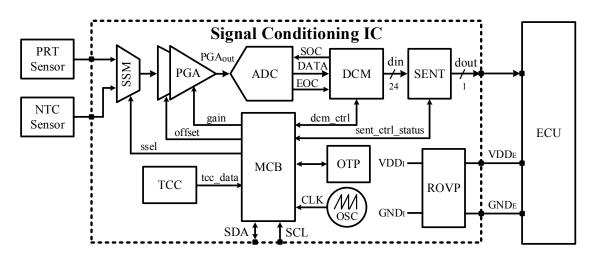
Figure 3. Signal conditioning IC for pressure and temperature sensors.
