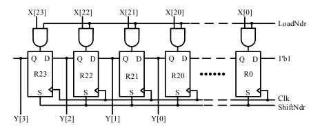
Figure 11. Nibble data register architecture.
