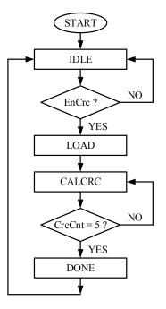
Figure 8. SENT CRC controller flow chart.
