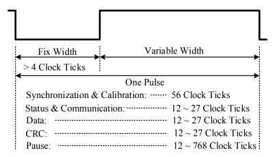
Figure 2. SENT pulse timing characteristics.
