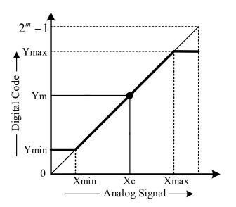
Figure 17. Transfer characteristics for measuring signal value.
