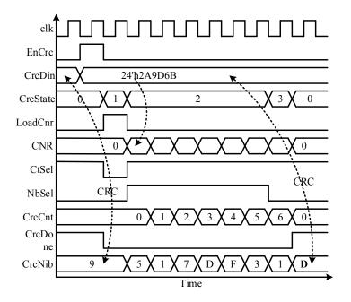
Figure 9. SENT CRC controller timing diagram.
