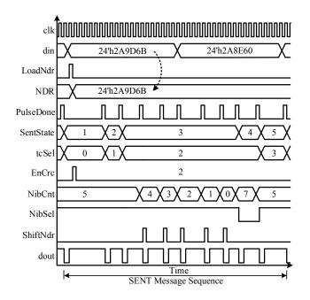
Figure 6. SENT main controller timing.
