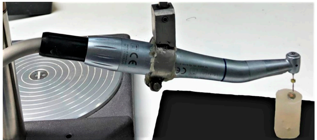
Figure 2. Standardized post space preparation with customized hand piece attached to dental surveyor.
