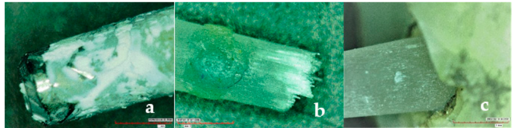
Figure 5. (a) Specimen with adhesive failure; (b) Specimen with cohesive failure; (c) Specimen with mixed type failure.
