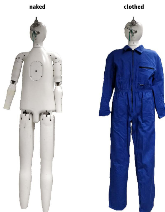
Figure A1. Determining the clothing insulation of the work coveralls used in our study using a thermal manikin.
