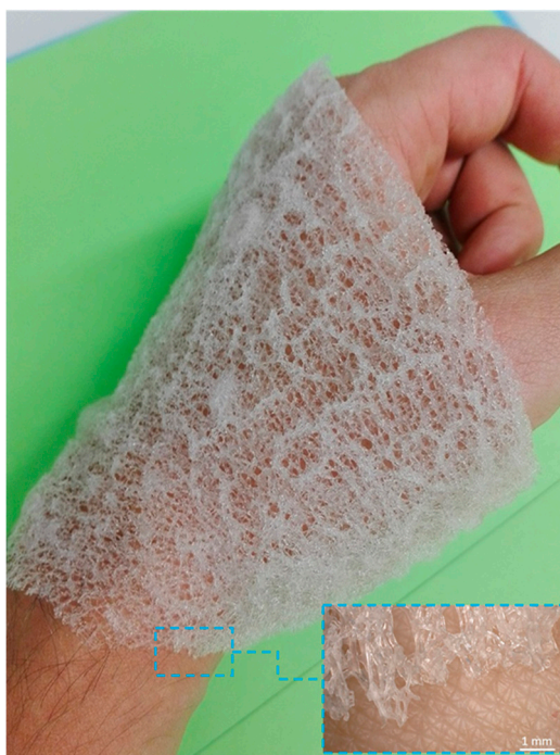
Figure 11. Gauze fabric-like morphology of chitinous scaffold isolated from I. labyrinthus . Such flexible biomaterial can be easily placed on the surface of human skin.
