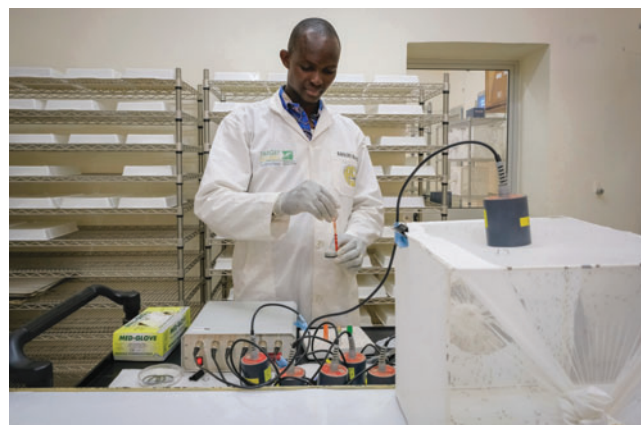
FIG. 3. Setting up of the Hemotek ® blood feeding system of mosquitoes (transgenic and wild type) in the ACL 2 insectary facility at the IRSS, Bobo-Dioulasso in Burkina Faso. Filling a membranous chamber with rabbit blood using a pipette. Mosquitoes suck the blood through a Parafilm ® membrane. The cage contains female mosquitoes engorged on the membrane-fed blood meal (Target Malaria © All rights reserved). Pictured: Roger Sanou (Deputy Insectary Manager). Color images are available online.
