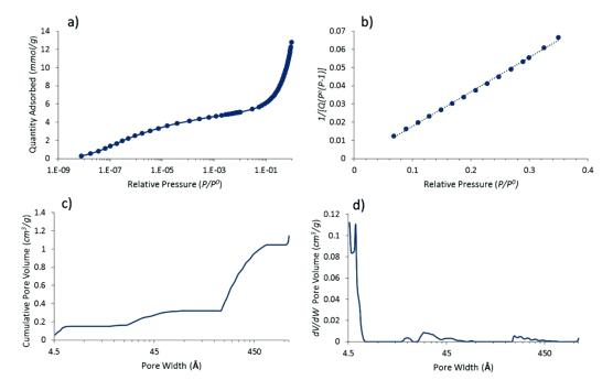
**Figure 3.** BET (77 K) nitrogen adsorption isotherm results for platinum nano-catalyst embedded in a microporous heterocarbon (Pt@cPIM): (**a**)  $N_2$  adsorption isotherm; (**b**) BET analysis plot; (**c**) cumulative pore volume; (**d**) pore width distribution (NLDFT (Non-Localised Density Functional Theory)) equilibrium for cylindrical pore model).
