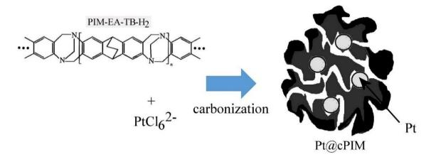
**Figure 1.** Molecular structure of PIM-EA-TB-H<sub>2</sub> and schematic depiction of the adsorption of hexachloroplatinic(IV) acid followed by mild vacuum carbonization to give a platinum nano-particle containing microporous heterocarbon.
