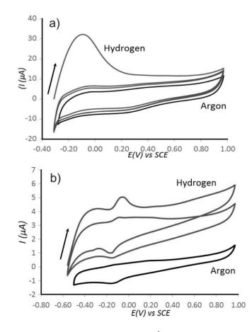
**Figure 5.** Cyclic voltammograms (scan rate 10 mV s<sup>-1</sup>) at Pt@cPIM immobilized onto a 3 mm diameter glassy carbon electrode immersed into (**a**) aqueous 0.1 M HClO<sub>4</sub> and (**b**) aqueous 10 mM PBS pH 7 solution purged with Ar or H<sub>2</sub>.
