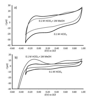
**Figure 6.** Cyclic voltammograms (3rd cycle) at Pt@cPIM immobilized onto a 3 mm diameter glassy carbon electrode immersed into Ar saturated 0.1 M HClO<sub>4</sub> without/with 1.0 M methanol recorded at a scan rate of (**a**) 100 mV s<sup>-1</sup> and (**b**) 10 mV s<sup>-1</sup>.
