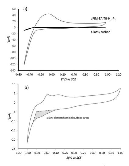
**Figure 4.** Cyclic voltammograms (3rd cycle, Ar saturated, scan rate  $10 \text{ mV s}^{-1}$ ) at Pt@cPIM immobilized onto a 3 mm diameter glassy carbon electrode immersed into (**a**) 0.1 M HClO<sub>4</sub> solution and (**b**) 10 mM phosphate buffer pH 7 solution with highlighted hydrogen electrochemical underpotential adsorption region (grey).
