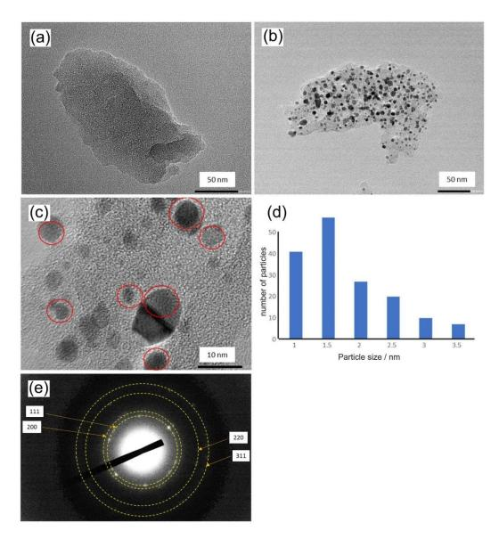
**Figure 2.** Transmission electron microscopy images for (**a**) carbonized hexachloroplatinate loaded polymer of intrinsic microporosity (PIM-EA-TB-H<sub>2</sub>), (**b**) carbonized PIM-EA-TB-H<sub>2</sub> with embedded nano-platinum, (**c**) high magnification micrograph showing platinum crystal lattice planes, (**d**) particle size distribution analysis, and (**e**) electron diffractogram with characteristic *hkl* reflections for platinum face-centered cubic phase.
