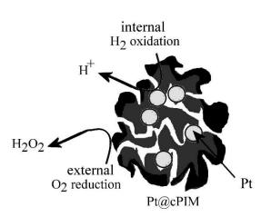
**Figure 8.** Schematic depiction of the catalytic process involving hydrogen and oxygen to give hydrogen peroxide.
