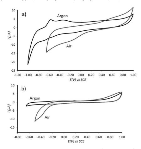
**Figure 7.** Cyclic voltammogram (3rd cycle, scan rate (**a**) 10 mV s<sup>-1</sup> and (**b**) 5 mV s<sup>-1</sup>) for oxygen reduction at Pt@cPIM immobilized onto a 3 mm diameter glassy carbon electrode immersed into 10 mM phosphate buffer solution pH 7 purged with either Ar or air.
