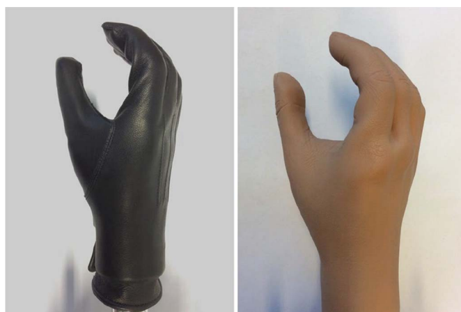
Figure 2. The Hűfner hand was commonly used with a leather glove applied (left). With a contemporary cosmetic glove (right), the Hűfner hand looks similar to a standard myoelectric or body-powered hand.
