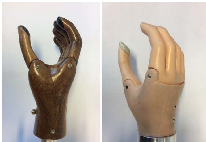
Figure 1. Original wooden Hűfner hand (left) and plastic Hűfner hand (right). The pawl of the locking mechanism can be seen on the palm side.
