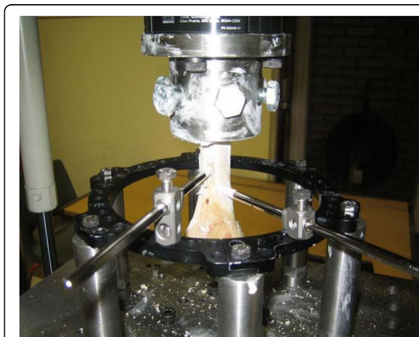
Figure 1 A typical test setup using half pins. The bone is held by the mount at the top end of the test frame and the ring is held rigidly by the bottom end of the frame. The weakest link in the setup is wires or pins connecting the bone to the rings. When load is applied to the bone from the top end it will displace depending on how rigidly it is held by wires or pins.
