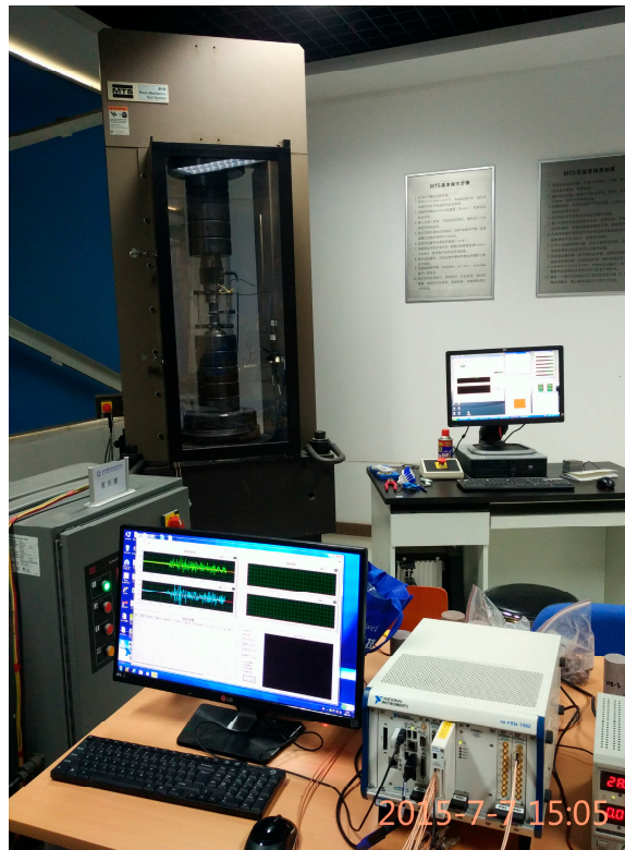
Figure 3. MTS 815 servo-controlled hydraulic testing machine for the laboratory tests.
