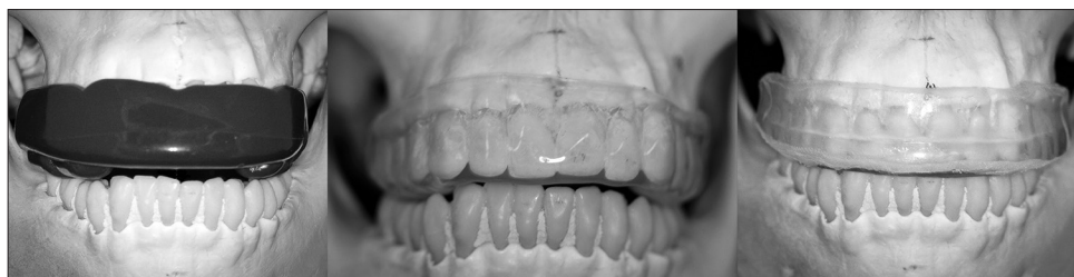
Figure 1: Over the counter (left), custom (middle), and novel (right) mouthguard on anatomical skull model
