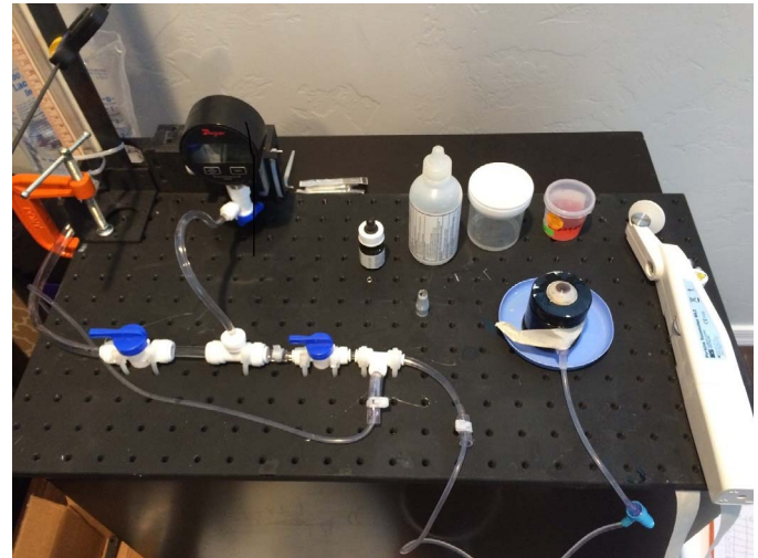
Figure 6. Experimental set up for cadaver eye IOP comparison.
