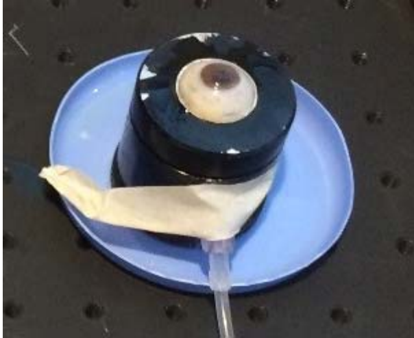
Figure 4. Ocular globe stabilizing apparatus for measuring IOP.
