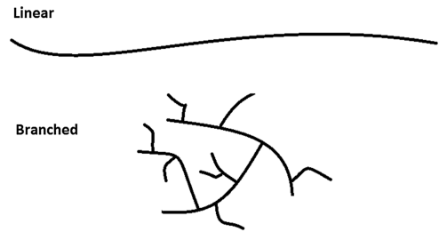
FIGURE 1. Linear versus branched polymers. Drawings representing linear and branched polysaccharides. The volume "swept out" by a fully extended linear fiber is much greater than a fiber with an equal number of sugar units (same molecular weight) but with a "bush-like," highly branched configuration. Because the volume occupied by a polymer molecule is a function of the radius cubed, even small increases in effective hydrodynamic size can translate into a large increase in viscosity for linear fibers.
