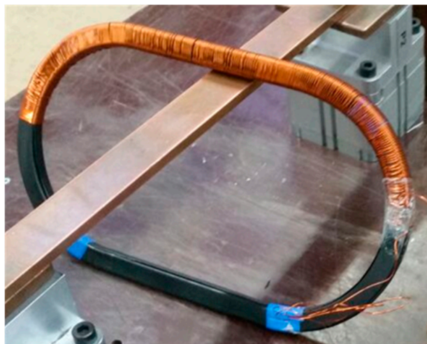
Figure 1. Current transformer core with partially distributed secondary winding.
