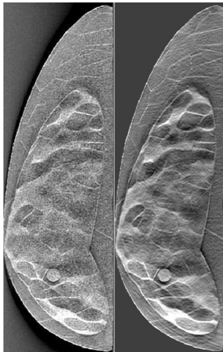
Figure 4. An unfiltered DBT image (left) of a 25% dense phantom and the same image after application of the Wiener filter (right). The unfiltered image was acquired across a 60^\circ span with 15 projections.
