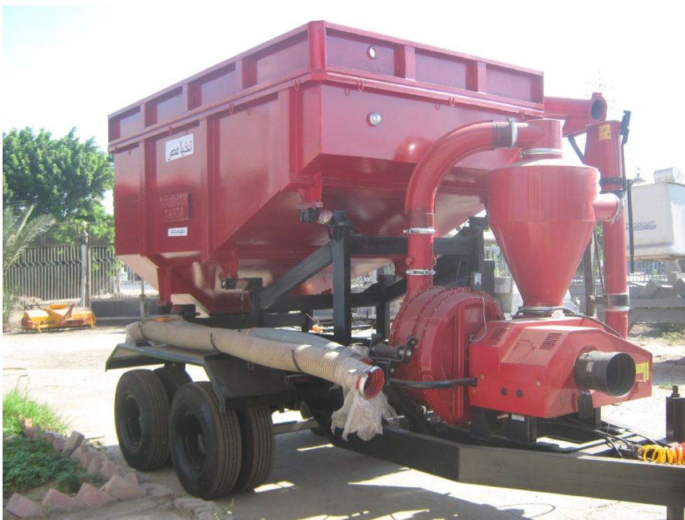
Figure 1. Photo of the developed grain cart for wheat transportation.
