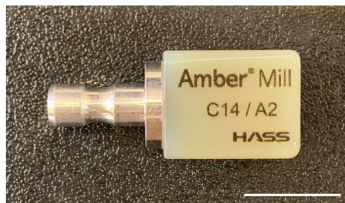
Figure 5. A bar-shaped lithium disilicate block (Amber Mill, HASS Co., Gangneung, Korea). This rectangular block is 14 mm in height, and is available for single restorations. Bar = 1 cm.
