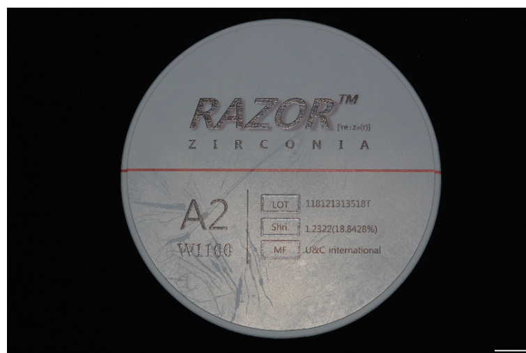
Figure 4. A disc-shaped zirconia block (Razor, U&C International Co., Ltd., Seoul, Korea). This block is partially sintered and 98 mm in diameter, and is available for a full arch implant-supported restoration. Bar = 1 cm.
