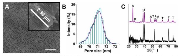
Figure 1. Structures of TiO<sub>2</sub> nanotubes on titanium (Ti-NTs). (A) SEM images of the Ti-NTs. Inset: cross-section view. Scale bar, 500 nm. (B) Pore size distribution of Ti-NTs determined by Nano Measurer. Error bars denote the standard deviations over triplicate measurements with the same implants. (C) XRD pattern of Ti-NTs before (bottom) and after (top) annealing treatment. A: anatase, R: rutile, and T: amorphous.
