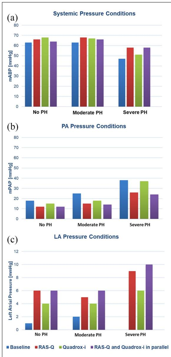
**Figure 4.** Pressure measurements comparing the performance of RAS-Q<sup>®</sup> with Quadrox-i<sup>®</sup> in a single animal. PH: pulmonary hypertension; mABP: mean arterial blood pressure; PA: pulmonary artery; mPAP: mean pulmonary artery pressure; LA: left atrial.
