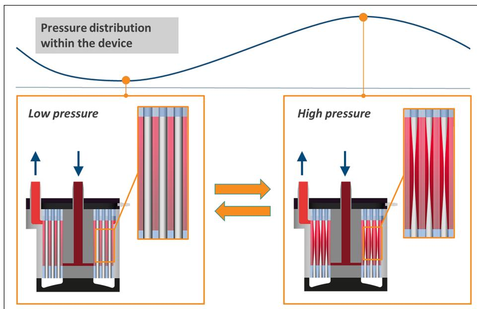
**Figure 1.** Schematic overview of RAS-Q<sup>®</sup> technology illustrating the effect of different pressures on the compliance elements (silicone tubes) placed within the polymethylpentene fiber bundle. Copyrights © 2018 enmodes. All rights reserved. This image is not covered by the terms of the Creative Commons license of this publication. For permission to reuse, please contact the rights holder.
