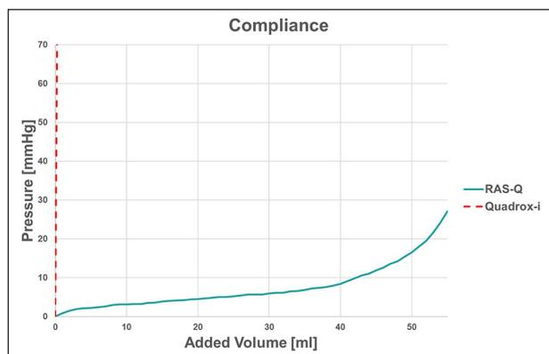
**Figure 2.** Compliance measurement illustrating the effect of the integrated silicon tubes.
