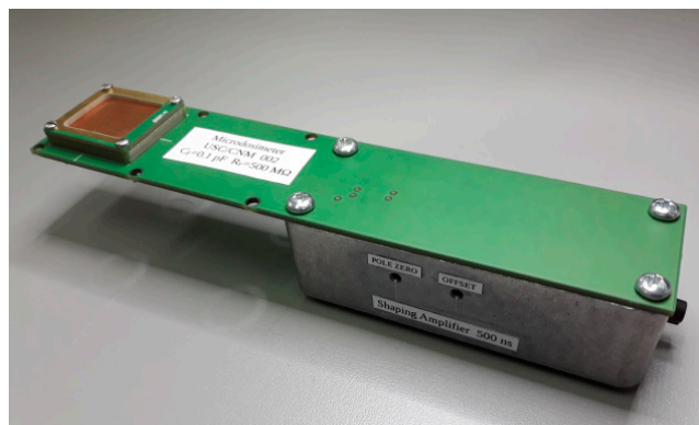
Figure 9. Photograph of a 3D-cylindrical microdetector setup. The dimensions of the setup (170 × 35 mm) make it a portable system. Image taken from [39].
