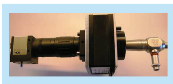
Figure 3. Hyperspectral laparoscopic system consisting in a charged-coupled device camera and a liquid crystal tuneable filter attached to a regular rigid laparoscope.
