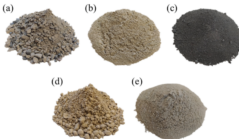
Fig. 2. Experimental materials, (a)Gangue, (b)Fly ash, (c) Gasification coarse slag, (d) Desulfurization gypsum, (e) Cement.
