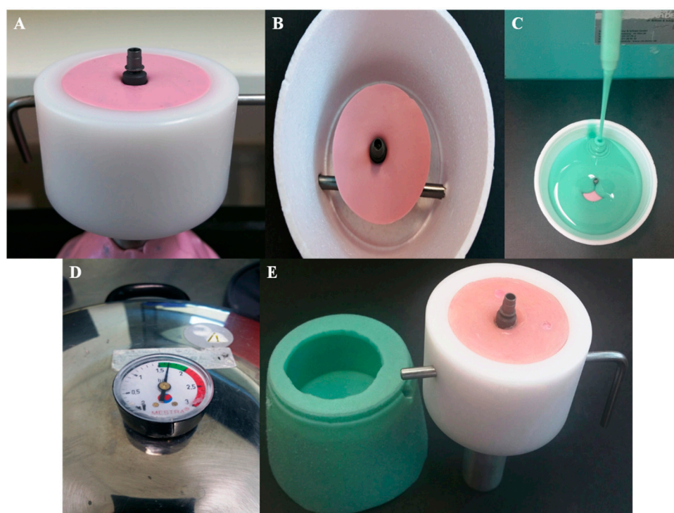
Figure 2. Fabrication of the sample cup holder for fatigue testing; (A) implants were screwed into heavy putty (Coltene whaledent, Altstätten/Switzerland). (B) Ti-Base abutment torqued to implant and ready to pour duplicate material. (C) Silicone duplicate material (Exaktosil N21, Bredent) poured into the cup. (D) Silicone replica put to set in a pressure pot to avoid porosity. (E) Silicone replica of the sample cup with the implant and Ti-Base abutment inverted and acrylic resin (Palapress vario, Heraeus Kulzer Wehrheim, Germany) poured in the mold and checked in the original chewing simulation sample cup for fitting.
