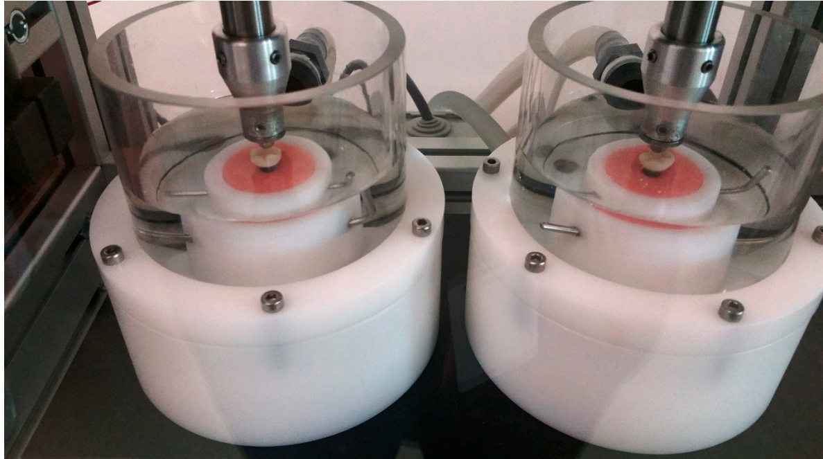
Figure 3. Crowns undergoing thermal cycling in a chewing simulator during fatigue testing.
