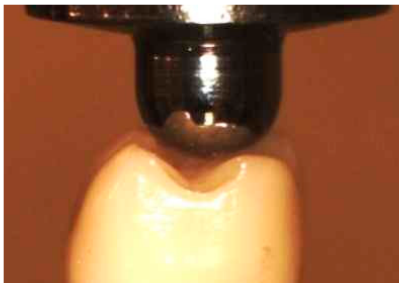
Figure 4. Position of the indenter during the compressive testing.
