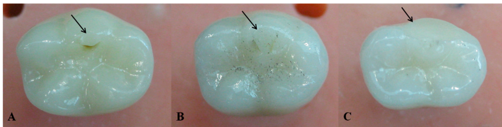
Figure 5. Wear facets at the indenter occlusal contact upon completion of the chewing simulation (arrows). (A) Milled lithium disilicate veneer, (B) hand-layered veneer, and (C) arrow indicating the chipping on the disto-buccal cusp at the indenter occlusal contact during chewing simulation.
