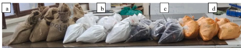
Fig. 1. Red pepper pod samples packed in different storage materials, a = jute sacks, b = PICS bags, c = fertilizer liner sheet (FLS), d = fertilizer-woven polypropylene + liner sheet.
