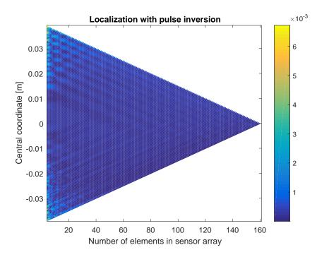
**Figure 11.** Color-coded plot of the difference between the exact defect location and the location obtained when applying the direct linear approach using sensor arrays with varying numbers of elements and centered at different coordinates. The results were obtained using the second harmonic signals emitted by the defect, with the use of pulse inversion.
