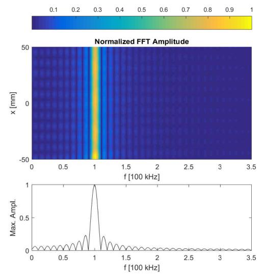
**Figure 3.** (Top) Frequency spectra of the calculated normal displacement signals for a number of points on the top surface of the plate, with x-coordinates ranging from -50 mm to 50 mm. (Bottom) Normalized maximum FFT amplitude response measured along the top surface of the plate.
