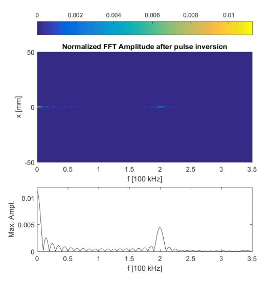
**Figure 4.** (Top) Frequency spectra obtained after applying the pulse inversion technique on the calculated normal displacement signals for a number of points on the top surface of the plate, with x-coordinates ranging from -50 mm to 50 mm. (Bottom) Normalized maximum FFT amplitude response measured along the top surface of the plate, after applying the pulse inversion technique. The figures clearly illustrate the generation of a second harmonic at the position of the crack (x = 0).
