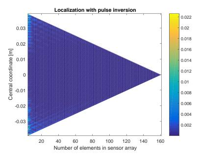
**Figure 13.** Color-coded plot of the difference between the exact defect location and the location obtained when applying the direct quadratic approach using sensor arrays with varying numbers of elements and centered at different coordinates. The results were obtained using the second harmonic signals emitted by the defect, with the use of pulse inversion.
