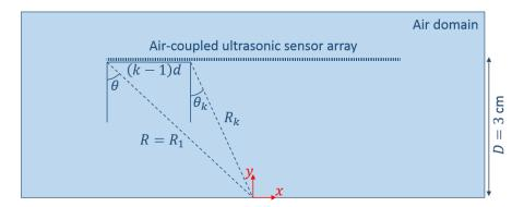
Figure 6. Representation of the near-field situation used in the beamforming algorithms.
