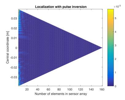
**Figure 9.** Color-coded plot of the difference between the exact defect location and the location obtained when applying the sum-and-delay approach using sensor arrays with varying numbers of elements and centered at different coordinates. The results were obtained using the second harmonic signals emitted by the defect, with the use of pulse inversion.
