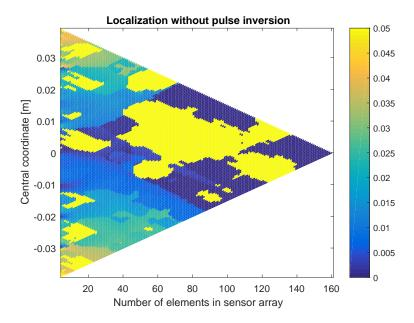
**Figure 8.** Color-coded plot of the difference between the exact defect location and the location obtained when applying the sum-and-delay approach using sensor arrays with varying numbers of elements and centered at different coordinates. The results were obtained using the second harmonic signals emitted by the defect (without using pulse inversion). Saturated yellow regions mean that the determined location is equal to or more than 5 cm away from the exact defect location.
