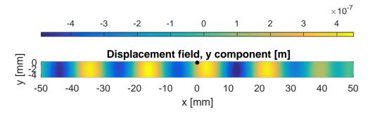
**Figure 2.** Snapshot of the calculated *y*-component of the displacement field in the aluminum sample, clearly illustrating the presence of an  $A_0$  guided Lamb wave. The black dot indicates the location of the near-surface crack.
