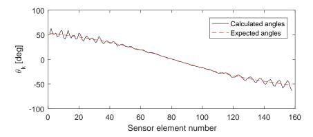
**Figure 12.** Angle  $\theta_k$  versus sensor element number of the first of four successive sensors at which the wave impinges. The solid black line corresponds to the angles calculated using the direct quadratic approach. The dashed red line corresponds to the angles that are theoretically expected.
