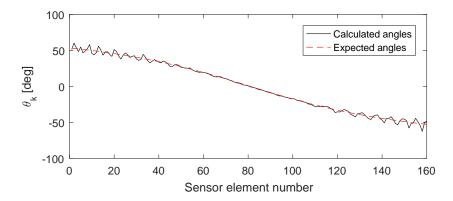
**Figure 10.** Angle  $\theta_k$  versus sensor element number of the first of two successive sensors at which the wave impinges. The solid black line corresponds to the angles calculated using the direct linear approach. The dashed red line corresponds to the angles that are theoretically expected.
