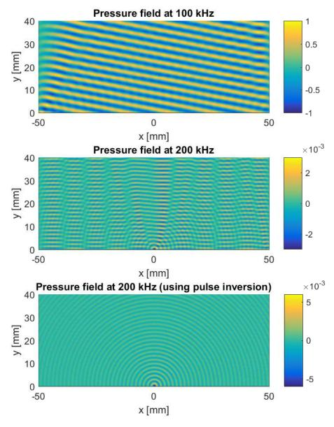
**Figure 5.** Radiation patterns in air above the aluminum plate with a near-surface crack. (Top) Fundamental frequency field showing no evidence of the presence of a crack. (Middle) Second harmonic field showing slight radiation of the harmonic into the air, starting from the crack position (x = 0). (Bottom) Second harmonic field obtained after applying the pulse inversion technique. The crack clearly behaves as a source of nonlinear emission.
