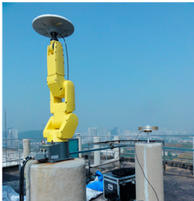
Figure 2. Robot antenna calibration facility at Wuhan University.
