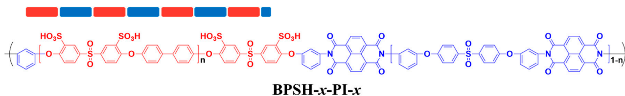
Figure 4. Representative chemical structures of sulfonated hydrocarbon-based block copolymers [63,64,67,68].
