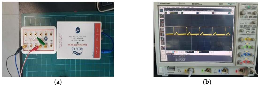
Figure 10. ECG performance tester for compliance tests with signal: (a) SECG 4.0; and (b) the signal extracted by SECG 4.0 using oscilloscope.
