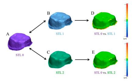
**Figure 7.** Simplified graphic representation of the analysis by best-fit alignment, **A**, Scan data of the gypsum model by laboratory scanner, **B**, Scan data using the AEGIS intraoral scanner, **C**, Scan data using the CEREC intraoral scanner, **D**, Deviation after superimposition of A and B displayed in a color-coded map. **E**, Deviation after superimposition of A and C displayed in a color-coded map.
