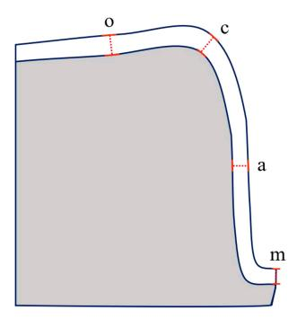
**Figure 5.** Schematic diagram of the points measured on each cross-section, o, occlusal gap (midpoint of occlusal wall); c, gap of cusp tip (axio-occlusal transition point); a, axial gap (midpoint of axial wall); m, marginal gap.
