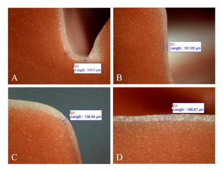
**Figure 6.** The blue lines represent the measurement discrepancies between the crown and the abutment tooth by the analysis software. **A**, marginal gap, **B**, axial gap, **C**, gap of the cusp tip, **D**, occlusal gap.
