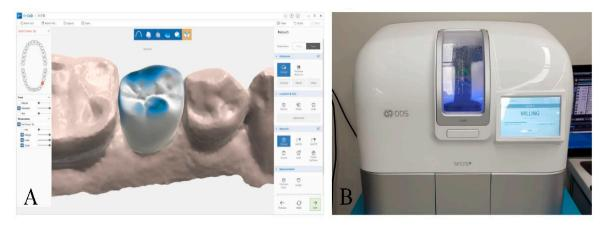
**Figure 4.** Chairside CAD/CAM procedures. **(A)** Planning a chairside crown with the design software. **(B)** Manufacturing a lithium disilicate crown with the milling machine.
