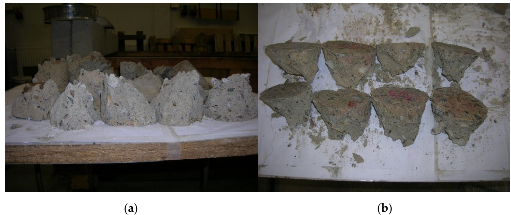
Figure 3. Concrete specimens after uniaxial compressive tests: (a,b) views of the form of failure.
