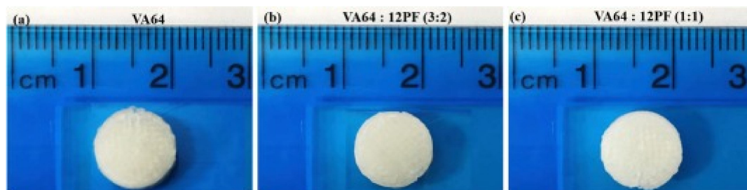
Figure 10. Pictures of ramipril printlets. (a) VA64, (b) VA64:12PF (3:2) and (c) VA64:PF12 (1:1). Image reproduced with permission from [78]. Copyright Elsevier, 2018.
