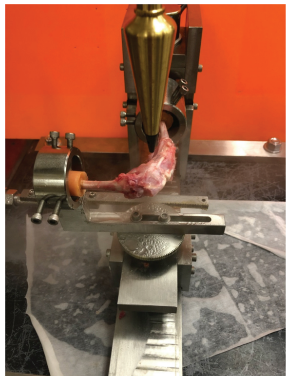
Figure 3. Joint contracture measurement setup demonstrating the custom rabbit-knee-gripping device placed within the MTS. The femoral insertion of the medial collateral ligament representing the axis of rotation is placed under the plumb bob.
