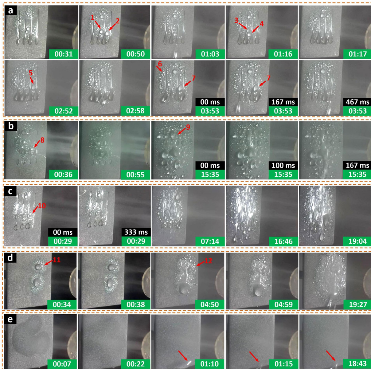
Figure 7. Fog harvest processes on different surfaces. Fog harvest processes that were carried out on the (a) superhydrophobic surface with wedge-shaped superhydrophilic dimple array, (b) superhydrophobic surface with round superhydrophilic dimple array, (c) superhydrophobic surface with connected round superhydrophilic dimple array, (d) bare superhydrophobic surface and (e) bare superhydrophilic surface. Dimension of the substrates was 40 \times 40 mm. Positions 1–12 marked by red arrows in (a–d) were some selected positions where the nucleated droplets were transported into the tracks. Dimensions of the patterns in (a–c) were illustrated in Fig. S2a–c, respectively in the Supplementary Information.
