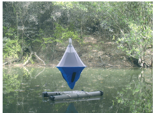
Fig. 2. – Floating biconical trap on the Comoe river, Burkina Faso.
