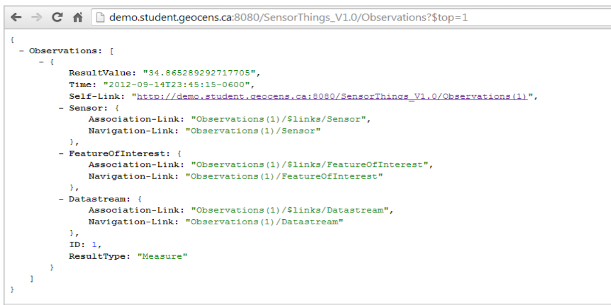
Figure A6. HTTP GET request and response to the OGC SensorThings through the Internet.
