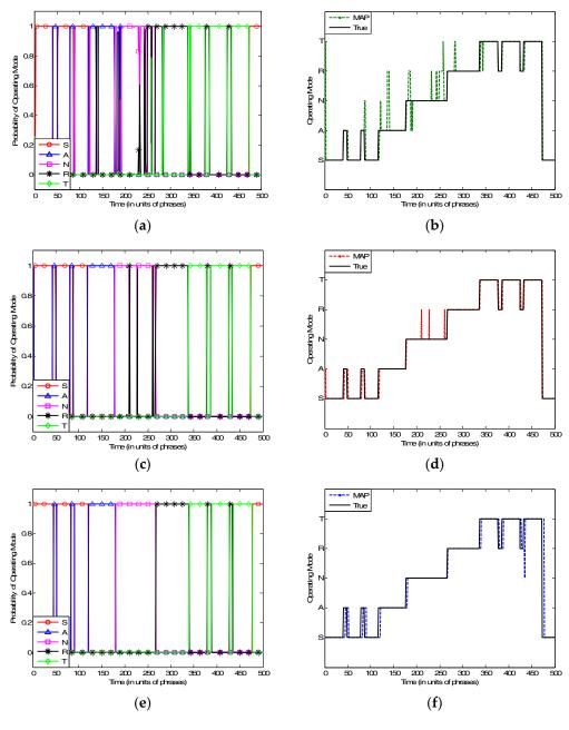
**Figure 4.** Recognition for MFR operating modes based on three recognition algorithms. (a) Probability distribution estimation based on HMM; (b) recognition based on HMM; (c) probability distribution estimation based on PSR and grid-filter; (d) recognition based on PSR and grid-filter; (e) probability distribution estimation based on PSR and proposed method; and (f) recognition based on PSR and proposed method.
