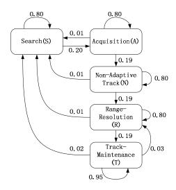
Figure 3. Operating mode transition of the MFR.
