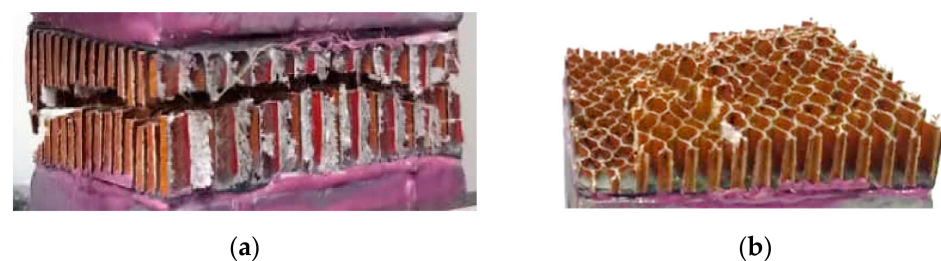
Figure 9. (a) Location of the fractured plane along the cell height, and (b) fractured surface of the polymer hexagonal HC core specimen, following the out-of-plane tensile loading.
